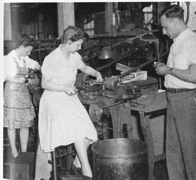
Betty Griffin and Mary Bragoni operate these hand edging machines, while Toolsetter Louis Ragazzino puts the gauge on a sample of the work. The girls are working on spring pins, and a careful checking to the close tolerances is important. This is real war work.
